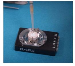
7. Drop the electrolyte onto the separator. Use only the amount of electrolyte necessary to impregnate the porous material. Avoid excess electrolyte. Typically, less than 50 µl of electrolyte is suitable.
