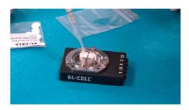
8. Drop the electrolyte onto the separator/electrodes. Use only the amount of electrolyte necessary to impregnate the porous material. Avoid excess electrolyte. Typically, around 30  $\mu$ l of electrolyte is suitable.
