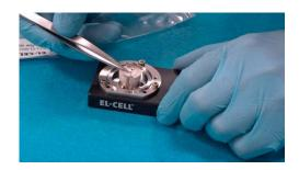
7. Make sure that the electrode strips are properly aligned before attaching the lid.
