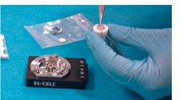
3. Put the electrode R, lithium metal in this case, on top of the piston.
