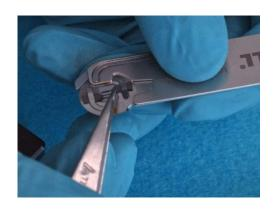
5. Turn the sample holder around and place the second electrode strip.
