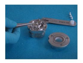
9. Attach the sample holder to the assembly. The markings 1 and 2 on the sample holder and cell base represent the electrodes. Use them as an aid for correct placement.
