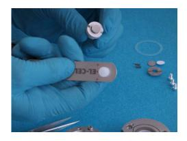
2. Use the loading tweezers to push the piston into the sleeve.
