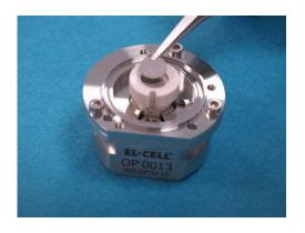
4. Put the R electrode disc, lithium metal in this case, on top of the piston.
