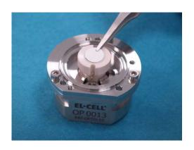
5. Put the separator on top. The separator must not be more than 10 mm in diameter. A smaller separator may be useful to prevent the sample holder from coming into contact with the electrolyte.
