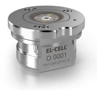
The PATCell-Opto-10 test cell is designed for operando characterization of electrodes using optical methods such as light microscopy or Raman spectroscopy in reflection mode.
