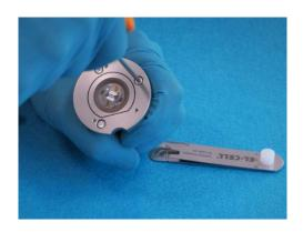
13. Finally fix the lid by using the Torx screws and the hexagon screwdriver 2.5mm.
