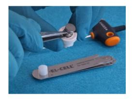
1. Assemble the lid as described above. Then insert the lower piston into the inner sleeve.
