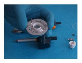
3. Insert the window thrust ring.
