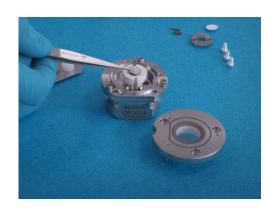
6. Put the R electrode disc, lithium metal in this case, on top of the piston.
