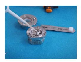
11. Drop the electrolyte onto the separator/electrodes. Use only the amount of electrolyte necessary to impregnate the porous material. Avoid excess electrolytes. Typically, less than 50 µl of electrolyte is suitable.
