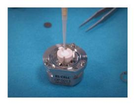
7. Drop the electrolyte onto the separator. Use only the amount of electrolyte necessary to impregnate the porous material. Avoid excess electrolytes. Typically, less than 50  $\mu$ l of electrolyte is suitable.
