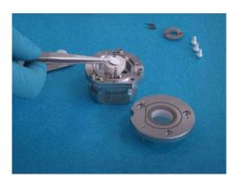
7. Put the separator on top. The separator must not be more than 10 mm in diameter. A smaller separator may be useful to prevent the sample holder from coming into contact with the electrolyte.
