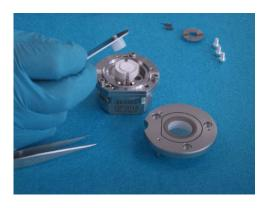
8. Use the loading tweezers again to press the cell stack further into the piston.
