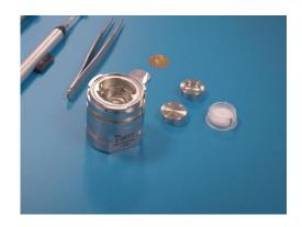
Put the insulation sleeve onto the worktop with the smaller side pointing upwards.
