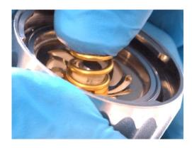
Check that the spring is seated correctly by bending it slightly in all directions.
