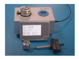
8. Insert the cell assembly into the PAT Socket of the PAT-Terminal-1.
