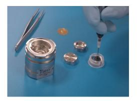
2. Insert the **lower electrode** into the sleeve with the active layer facing downwards.
