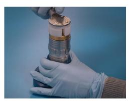
13. Attach the lid. Use the Screw cap torque wrench to tighten it until the set torque is reached.
