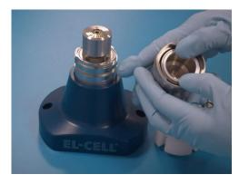
12. Insert a new sealing ring to the lid. For best tightness, use an aluminum seal.
