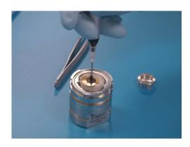
6. Insert the **upper electrode** into the insulation sleeve with the active layer facing downwards.
