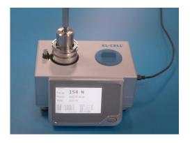
10. Use the provided torque controlled screw driver to adjust the force applied to the cell stack. The set force is shown on the display of the PATTerminal-1.
