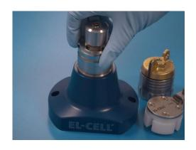
11. Remove the PAT-Cell-Force from the PAT-Terminal-1 and insert it into the cell assembly block for final steps.
