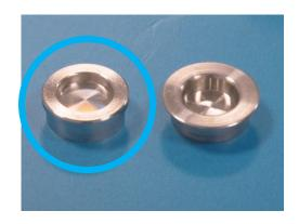
**Please note:** The PAT-Cell-Force uses a special version of the upper plunger with a smaller diameter, as seen in the image.
