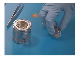
3. Attach the **lower plunger**. The lower plunger is available in different gap sizes to account for the thickness of the lower electrode and the separator used.
