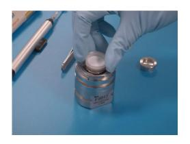
4. Align the contact spring of the sleeve with the horizontal contact pin inside the **cell base**. Then insert the assembly into the cell base.
