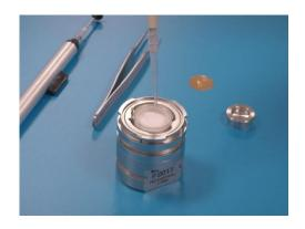
5. Evenly dispense approx. 100 µL of **electrolyte** on top of the separator with a pipette. Note: The optimum amount of electrolyte will depend on the thickness and porosity of the separator and the electrodes used.
