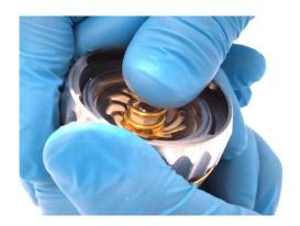
Now press the spring onto the pin until it touches the disc spring.
