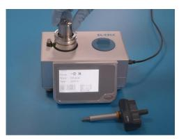
9. Attach the lid inset and turn it clockwise to lock it in place.
