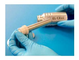
4. Remove the Ejector pin.
