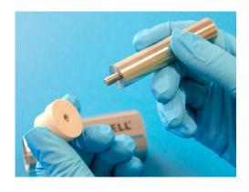
5 Unscrew the Ejector Ram from the Ejector pin.
