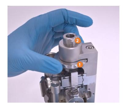
Turn the adjustment wheel 1 to change the force. You can read the approximate setting on the scale 2. When the lowest line on the scale is visible, the set force is approximately 1 N.
