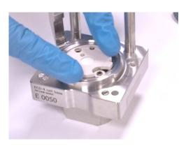
8. Insert the unit into the cell base. When properly aligned, the unit will slide into position easily. As a test, you should now be able to press the unit down with light force, and it should pop back a bit.
