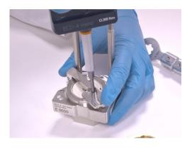
14.Continue to hold the lever in this position and gently tighten the clamping screw using the torque wrench supplied. Pay attention to the low tightening torque.
