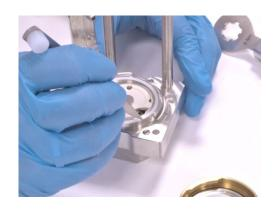
14. Flip the lever back up and insert a new PE sealing ring.
