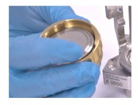
15.Insert the membrane into the screw cap. Be careful to touch the membrane only at the edge, not the center area.-
