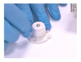
6. Now put on the thrust screw and tighten it by hand.
