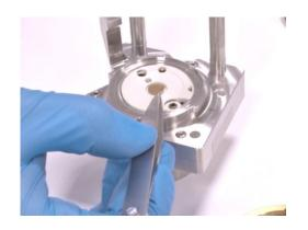
10.Place the working (upper) electrode on top of the glass frit. The active layer must point downwards.
