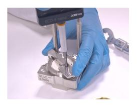
13.Continue to hold the lever in this position and gently tighten the clamping screw using the torque wrench supplied. Pay attention to the low tightening torque.
