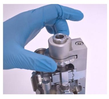
When the top line on the scale is reached, the set force is approximately 15 N.
