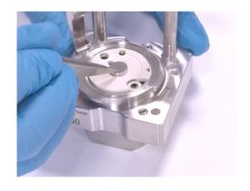
12.Insert the spacer disc. The spacer disc should completely cover the upper electrode.
