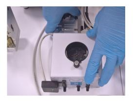
1. Plug the sensor cable (PAT-Channel to ECD-4-nano Sensor Box) into the female port of the ECD-4 Centering device.
