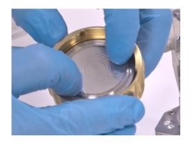
16.Press the membrane down slightly until it snaps into place. Be careful to touch the membrane only at the edge, not the center area. It should not fall out when you turn the lid upside down.
