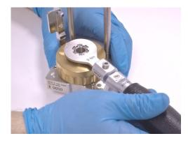
**17.** Put the screw cap on and tighten the centering thrust screw with the torque wrench until the tool releases.
