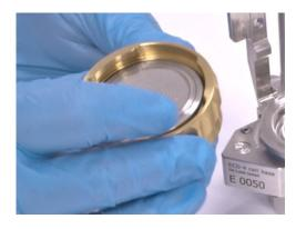
16. Insert the membrane into the screw cap. Be careful to touch the membrane only at the edge, not the center area.
