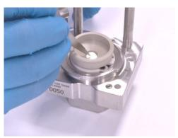
11. Place the upper electrode on top of the separator, with the active side pointing downwards.
