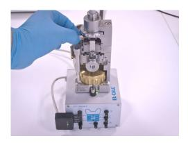
2. Insert the ECD-4-nano with attached sensor cable into the PAT-Stand-1.
