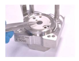
8. Place the lower electrode on top of the glass frit. The active layer must point upwards.
