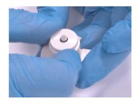
7. Now put on the thrust screw and tighten it by hand.
