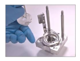
7. Use the provided tweezers to lift the frit flange out of the cell base.
