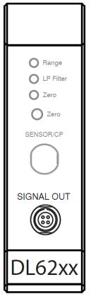
Signal output on controller, 4-pole male cable connector
