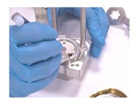
15.Flip the lever back up and insert a new PE sealing ring.
