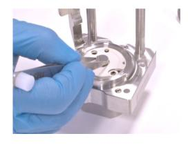
11.Insert the spacer disc. The spacer disc should completely cover the working electrode.
