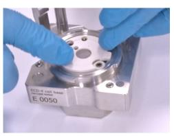
7. Insert the unit into the cell base. When properly aligned, the unit will slide into position easily. As a test, you should now be able to press the unit down with light force, and it should pop back a bit...
