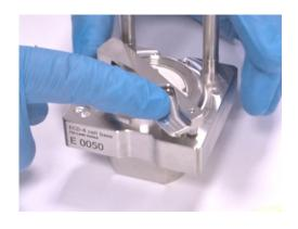
5. Fold the lever down to the stop and hold it in this position.
