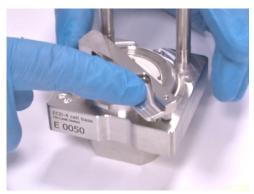
13. Fold the lever down to the stop and hold it in this position.
