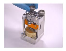
1. Put the device on an even surface and screw off the two knurled nuts.
