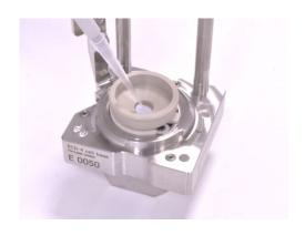
12.Add approx. 40 µl of electrolyte using a pipette.
