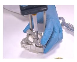
6. Continue to hold the lever in this position and gently tighten the clamping screw using the torque wrench supplied. Pay attention to the low tightening torque.
