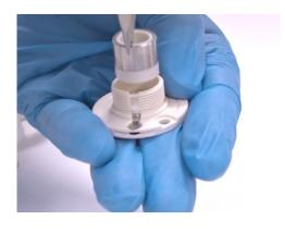
9. Remove the sleeve from the frit flange unit.
