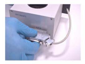
3. Plug the male connector into the Aux-in port of the PAT-Stand-1.
