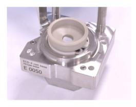
10. Place the Adjustment tool on the separator.
