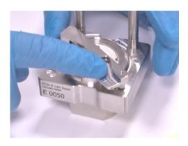
12.Fold the lever down to the stop and hold it in this position.
