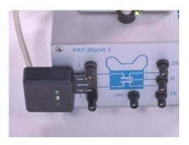
3. Change the sensor setting on the ECD-4-nano as explained at the beginning of this chapter. As soon as the middle LED on the Centering device lights up, the sensor is in the correct zero position (+/-20 µm). Lock the adjustment wheel. The ECD-4-nano is now calibrated.
