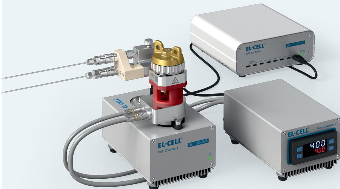
Complete PAT-Cell-Gas-HT setup with Temp-Controller-1 and PAT-Tester-x-8 potentiostat.
