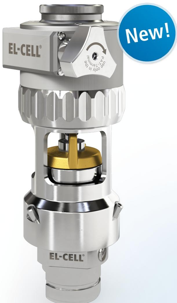
The PAT-Cell-Solid includes a built-in temperature sensor and, optionally, a gas pressure sensor and gas connections for flow-through operation. Its design ensures excellent sealing against the ambient atmosphere using proven metal lid seals and laser-welded electrode feed-throughs. Electrical connection is made without cabling by inserting the test cell directly into the PAT-Tester-x-8 potentiostat or PAT docking station, thereby preventing interference and simplifying operation.
