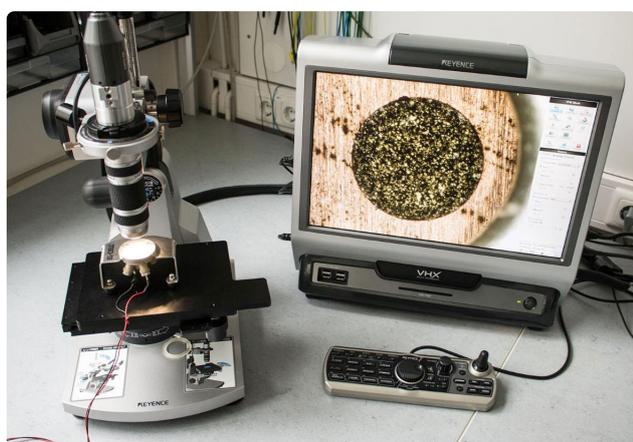
In this experiment, the ECC-Opto-Std test cell has been used to visualize the colour change of a graphite electrode during electrochemical lithiation. The microscope "looked" through the 1 mm diameter hole in the copper foil onto the backside of the graphite electrode.
