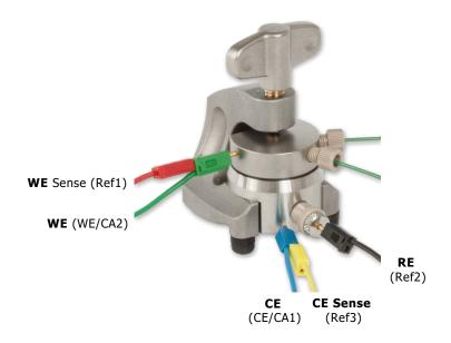
The notations in brackets refer to the standard connection with a Biologic potentiostat (MPG-2, SP, VSP and VMP series).
