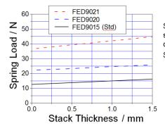
Spring load on stack vs. stack thickness for different springs. Standard is FED9015.
