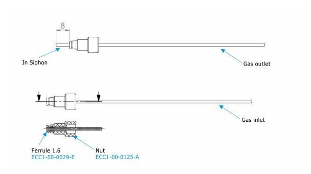
The provided fittings are compatible with 1/16 inch outer diameter tubing. We recommend the use of stainless steel or PEEKsil<sup>TM</sup> capillary tubing
