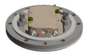
IV) Release the clamping claws (turn 90° counter clockwise) and remove the inner cell.
