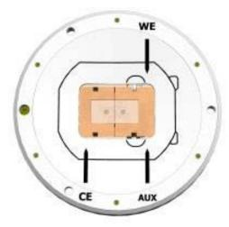
VI) Turn it upside down. Now you can see the two ram holders with the square rams, where the electrodes will be placed. Note the two nickel plated feed pins that will finally make the contact to these electrodes.
