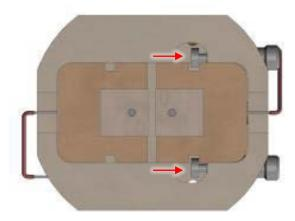
X) Place a rectangular piece of the glass fiber separator into the gap between the squared rams. The upper edge of the separator must have the same height like the ram holder, because the separator has to touch the glass window.
