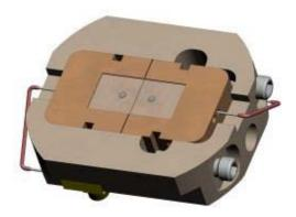
If the hight of the electrodes varies, you have different means to adjust the electrodes. There are 4 adjustment screws at the inner cell.
