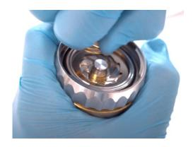
Remove the installed spring by pulling it off by hand. If it is stuck, it can also be loosened with a suitable tool (e.g., the back end of tweezers or a screwdriver).
