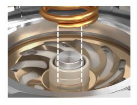
Position the new spring aligned with the high lug as shown in the image.
