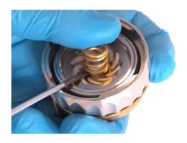
Remove the installed spring with a suitable tool (e.g., the back end of tweezers or a screwdriver). Be careful not to damage the PEEK part at the pin.
