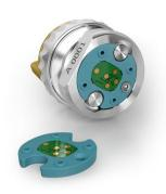
This upgrade kit can be used to retrofit an older PAT-Cell with a PAT-Button. The PAT-Button enables a PAT-Tester potentiostat to immediately recognize the inserted cell and display its ID and cell type.
