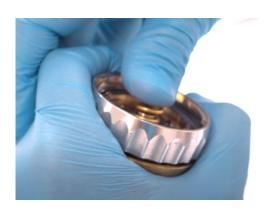
Now press the new spring evenly onto the pin until it touches the disc spring.
