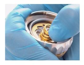
Check that the spring is seated correctly by bending it in all directions.
