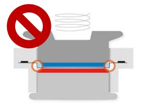
**Gap too large:** Excessive downward bending of built-in separator; reference ring is out of plane with separator.
