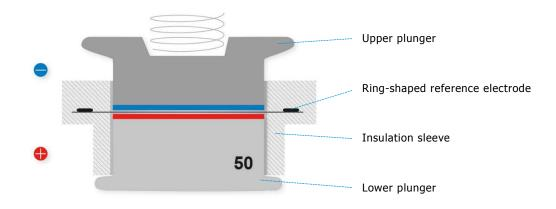
The lower electrode can have a thickness of up to 800  $\mu m$  provided that the proper gap size of the lower plunger is chosen. The maximum thickness of the upper electrode is 800  $\mu m.$
