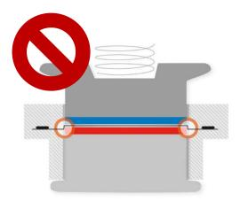
**Gap too small:** Excessive upward bending of built-in separator; reference ring is out of plane with separator.
