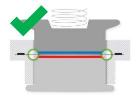
**Good case:** No bending of built-in separator; reference ring is in plane with separator.
