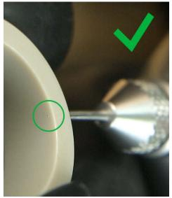
Pick up a small piece of lithium by a metal wire, and press the lithium into the feed-through hole of the REF sleeve until the lithium just arrives at the inner face of the sleeve, not less, not more. A dedicated tool,the ECC-RefLoad, is optionally available to ease this assembly step.)
