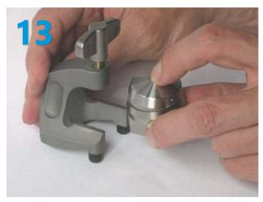
Insert the cell into the bracket by pressing down the lid while pushing the cell into the bracket.
