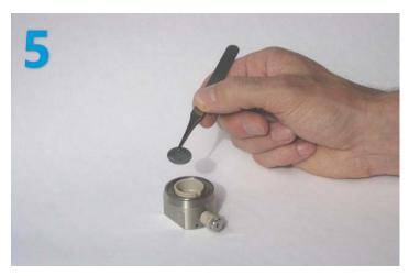
Place the 18 mm counter electrode into the sleeve.
