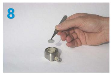
Place the working electrode, with its active layer downside, on top inside the sleeve.
