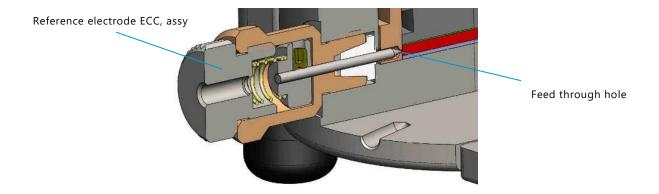
**Note**: By default, the REF sleeve comes with a 0.3 mm diameter bore. Depending on the reference or "wick" material used, it may be required to enlarge this bore. This can easily be done free-handed with the aid of a drill-bit. The REF bore diameter must not exceed 0.8 mm.
