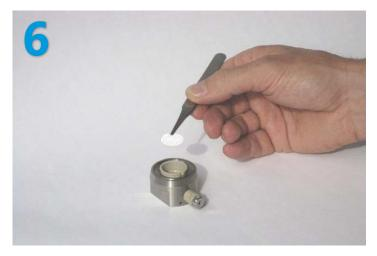
Put the glass fiber separator on top.
