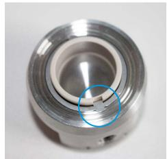
Mount the locking washer to align the side opening of the cell base with the feed-through hole of the REF sleeve.
