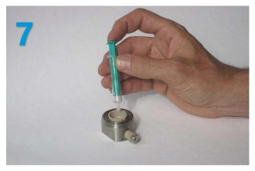
Dispense a defined amount of electrolyte onto the separator
