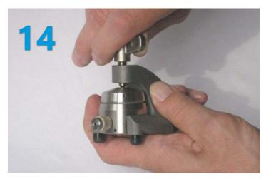
Tighten cell by turning the wing nut.
