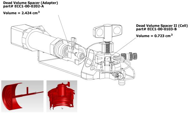
Visualised dead volume (both spacers installed = delivery condition = 3.024 cm<sup>3</sup>)
