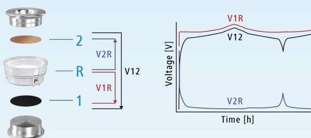
By monitoring the cell voltage and cell current of the battery, you can learn a lot about the performance and aging of the battery as a whole. However, a battery comprises two electrodes connected in series: cathode and anode.
