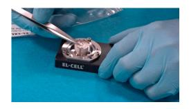
7. Ensure the electrode strips are correctly aligned before attaching the lid.
