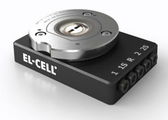
The ECC-Opto-10 test cell is designed for the operando characterization of electrodes using optical methods such as light microscopy or Raman spectroscopy in reflection mode.
