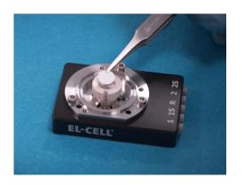
5. Put the separator on top. The separator must not exceed 10 mm in diameter. A smaller separator may be beneficial in preventing the sample holder from coming into contact with the electrolyte.
