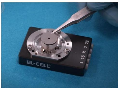
11. Put the holed current collector on top. Select the hole size according to the magnification used by the microscope.
