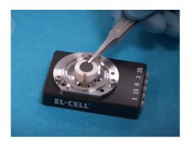
8. Put the self-standing electrode on top. If the electrode has a grid-like current collector, the grid must point downward toward the separator.
