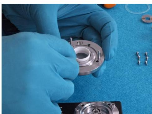
3. Insert the window thrust ring.
