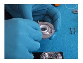
3. Insert the window thrust ring.
