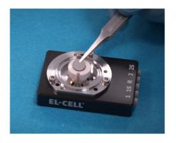
4. Put the electrode R, lithium metal, in this case, on top of the piston.
