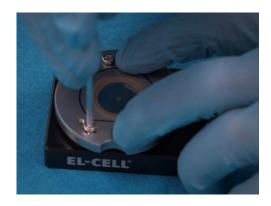
14. Finally, screw the cover on with the 2.5 mm hexagon screwdriver.
