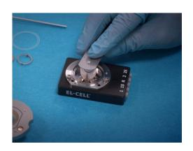
9. Push down the electrode stack using the loading tweezer.
