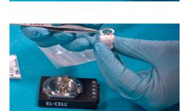
5. Attach the sample holder and press it down.
