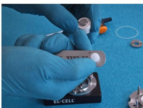
2. Use the loading tweezer to push the piston into the sleeve.
