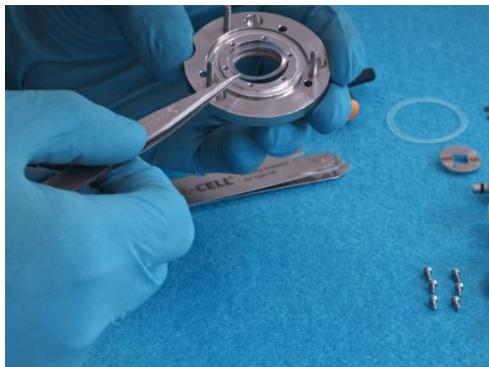
1. Turn the lid upside down. Insert the foil sealing into the lid.
