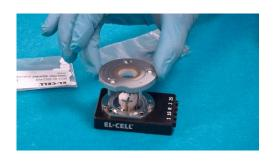
10. Put on the cell lid. Make sure that the flat side of the cell base and the straight line on the lid are parallel.
