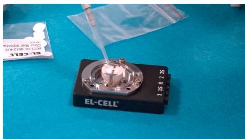
8. Drop the electrolyte onto the separator/electrodes. Use only the amount of electrolyte necessary to impregnate the porous material. Avoid excess electrolytes. Typically, around 30  $\mu$ l of electrolyte is suitable.
