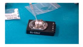
8. Drop the electrolyte onto the separator/electrodes. Use only the amount of electrolyte necessary to impregnate the porous material. Avoid excess electrolytes. Typically, around 30 µl of electrolyte is suitable.
