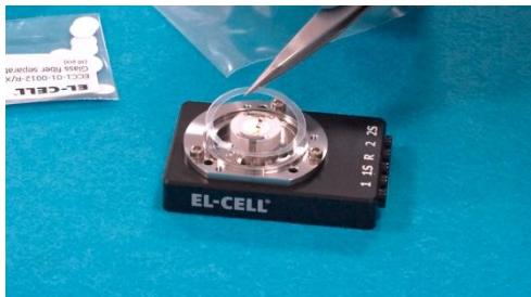
9. Insert the PE foil seal.
