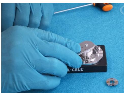
6. Use the loading tweezer again to push the cell stack further down.
