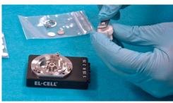
3. Put the electrode R, lithium metal, in this case, on top of the piston.
