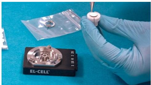
4. Put the separator on top and push it down using the loading tweezer.
