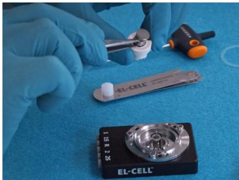
1. Follow the lid assembly steps. Then insert the lower piston into the inner sleeve.
