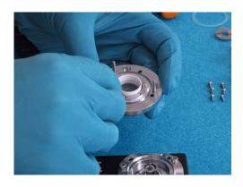
3. Insert the window thrust ring.
