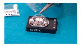
9. Insert the PE foil seal.
