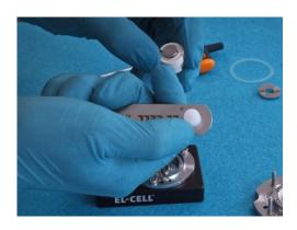
2. Use the loading tweezer to push the piston into the sleeve.
