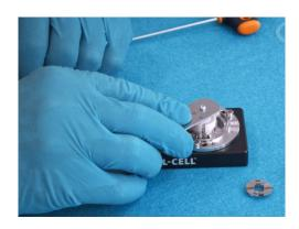
6. Use the loading tweezer again to push the cell stack further down.
