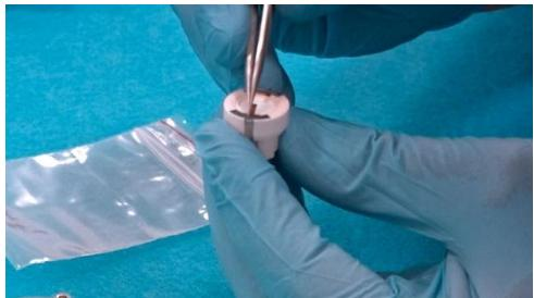
6. Insert the assembly into the cell base.
