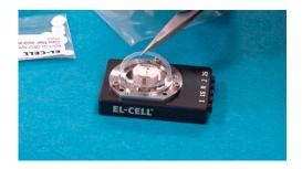
9. Insert the PE foil seal.
