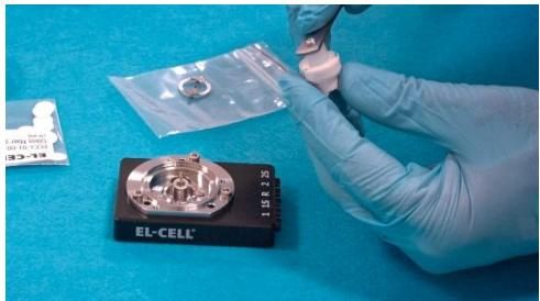
5. Attach the sample holder and press it down.
