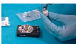
4. Put the separator on top and push it down using the loading tweezer.
