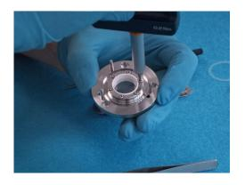
4. Attach the window flange and screw in the screws using the torque screwdriver 0.2 Nm.
