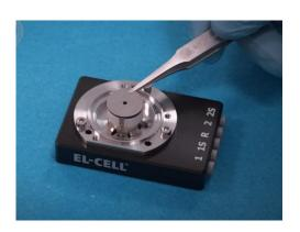
11. Put the holed current collector on top. Select the hole size according to the magnification used by the microscope.
