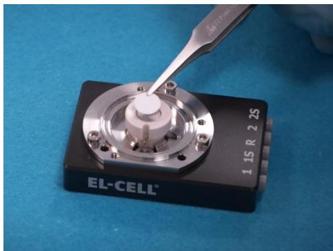
5. Put the separator on top. The separator must not exceed 10 mm in diameter. A smaller separator may be beneficial in preventing the sample holder from coming into contact with the electrolyte.
