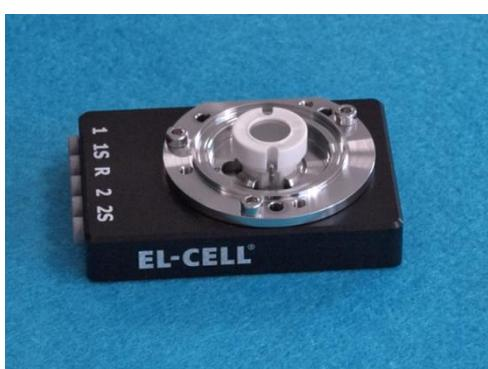
3. Place the assembly into the cell base.
