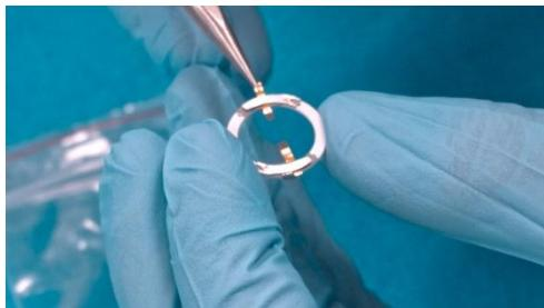
1. Assemble the lid as described above. Then attach the electrode strips to the sample holder.
