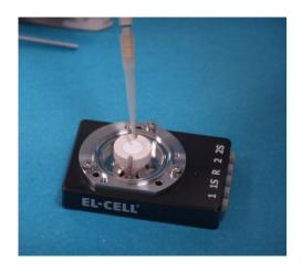
7. Drop the electrolyte onto the separator. Use only the amount of electrolyte necessary to impregnate the porous material. Avoid excess electrolytes. Typically, less than 50  $\mu$ l of electrolyte is suitable.
