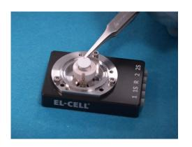
5. Put the separator on top. The separator must not be more than 10 mm in diameter. A smaller separator may be useful to prevent the sample holder from contacting the electrolyte.
