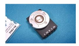
12. The ECC-Opto-10 is now ready for testing. It can now be removed from the glove box.
