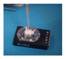
7. Drop the electrolyte onto the separator. Use only the amount of electrolyte necessary to impregnate the porous material. Avoid excess electrolyte. Typically, less than 50  $\mu$ l of electrolyte is suitable.
