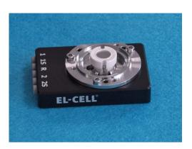
3. Place the assembly into the cell base.
