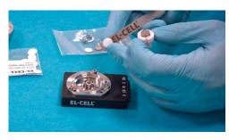
2. Use the loading tweezer to push the piston into the sleeve.
