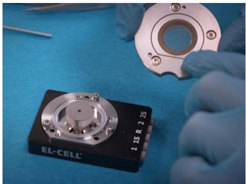
13. Put on the cell lid. Make sure that the flat side of the cell base and the straight line on the lid are parallel.
