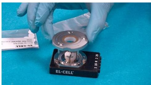
10. Put on the cell lid. Make sure that the flat side of the cell base and the straight line on the lid are parallel.
