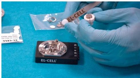
2. Use the loading tweezer to push the piston into the sleeve.
