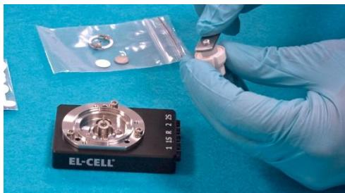
3. Put the electrode R, lithium metal, in this case, on top of the piston.
