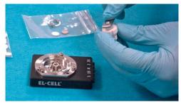
2. Use the loading tweezer to push the piston into the sleeve.
