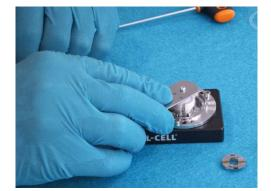
I-CELL BI-CELL 6. Use the loading tweezer again to push the cell stack further down.
