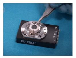
8. Put the self-standing electrode on top. If the electrode has a grid-like current collector, the grid must point downward toward the separator.
