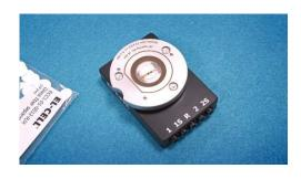
12. The ECC-Opto-10 is now ready for testing. It can now be removed from the glove box.
