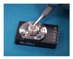
1. Follow the lid assembly steps. Then insert the lower piston into the inner sleeve.
