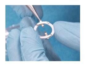
5. Attach the electrode strips to the sample holder.
