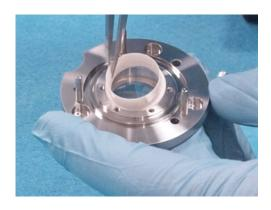
3. Insert the window thrust ring.
