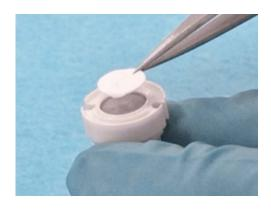
4. Put the separator on top. The separator must not be more than 10 mm in diameter. A smaller separator may be useful to prevent the sample holder from coming into contact with the electrolyte.
