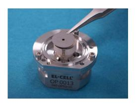
11. Put the holed current collector on top. Choose the hole size depending on the magnification used by the microscope.
