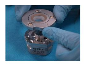
13. Put on the cell lid. Make sure that the flat side of the cell base and the straight line on the lid are parallel.
