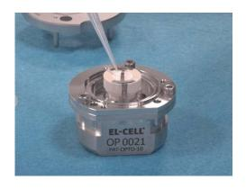
8. Drop the electrolyte onto the separator/electrodes. Use only the amount of electrolyte necessary to impregnate the porous material. Avoid excess electrolytes. Typically, less than 50 µl of electrolyte is suitable.
