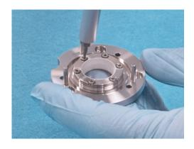
4. Attach the window flange and screw in the screws using the torque screwdriver 0.2 Nm.
