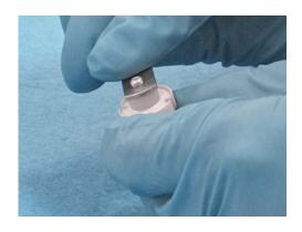
2. Use the loading tweezers to push the piston into the sleeve.
