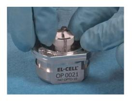
7. Insert the assembly into the cell base.
