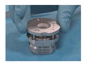
10. Ensure the electrode strips are correctly aligned before attaching the lid. Then put on the cell lid. Make sure that the flat side of the cell base and the straight line on the lid are parallel.
