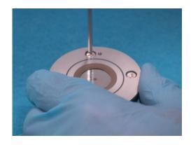
14. Finally, screw the cover on with the 2.5 mm hexagon screwdriver.
