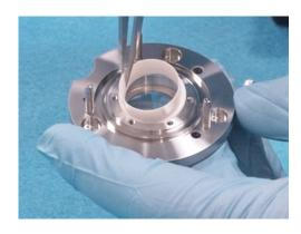
3. Insert the window thrust ring.
