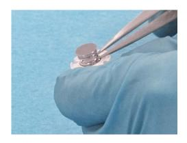
1. Assemble the lid as described above. Then insert the lower piston into the inner sleeve.
