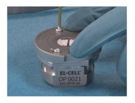
11. Double-check the proper alignment of the electrode strips.
