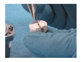
6. Attach the sample holder to the piston assembly.
