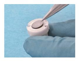
3. Put the electrode R, lithium metal in this case, on top of the piston.
