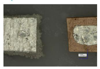
Lithium metal electrodes embedded into a glass fiber separator soaked with electrolyte. Applying a current of 20  $\mu A$  for 5 hours makes the lithium to dissolve from the supporting copper foil (right electrode) and to plate as dendrites on the opposite side (left electrode).
