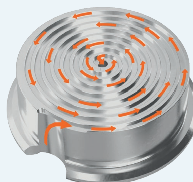
Gas flow along the surface of the lower plunger
