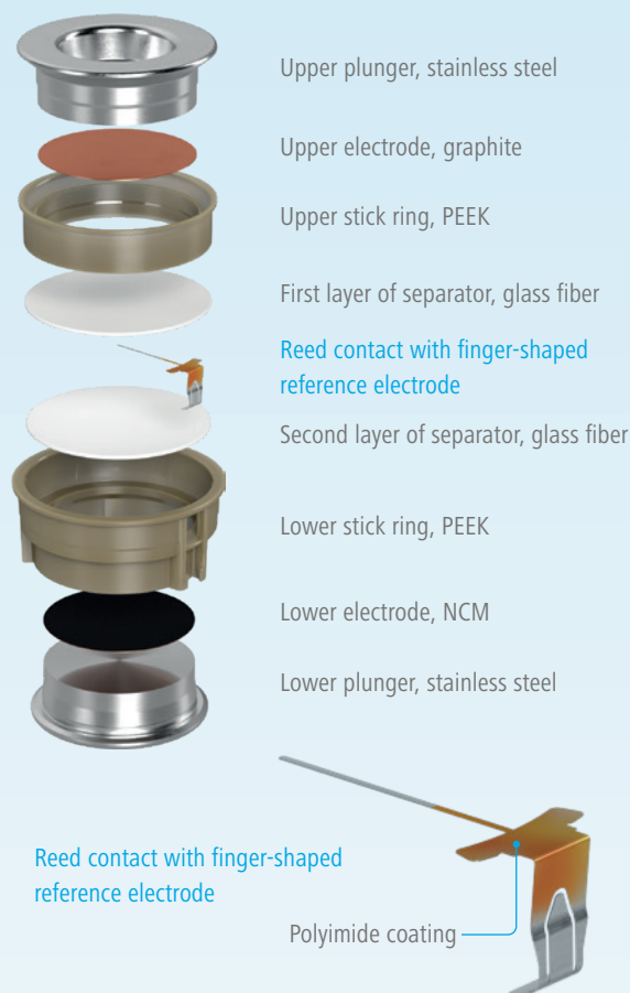
PAT-Core with finger-shaped reed contact
