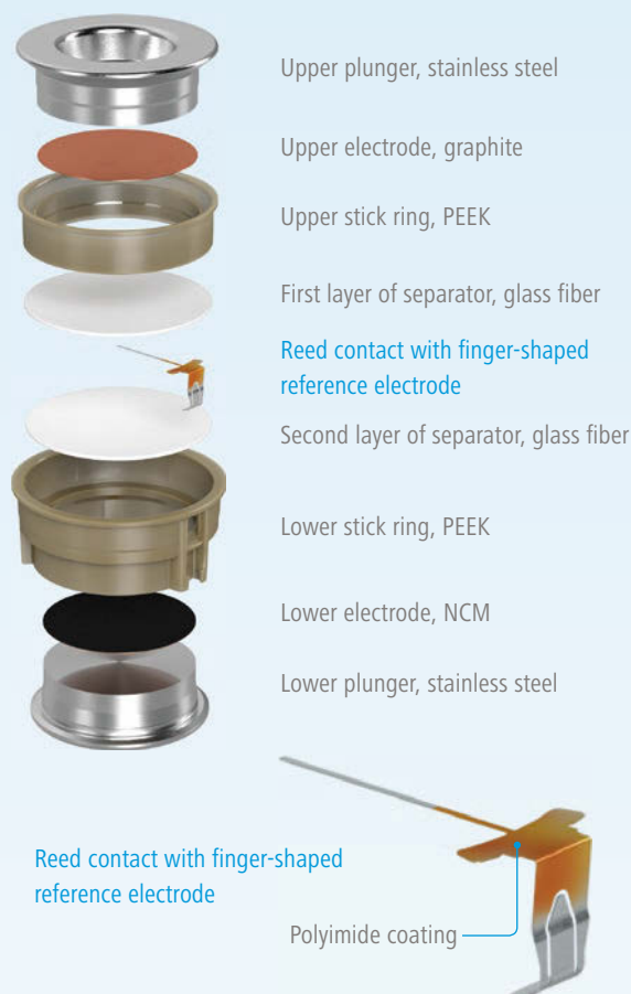
PAT-Core with finger-shaped reed contact
