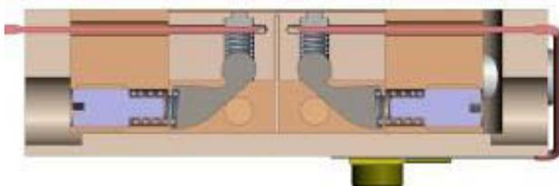
2. The two bigger adjustment screws serve to adjust the distance and parallelism between the two electrodes aka the width of the electrolyte (separator) gap.
