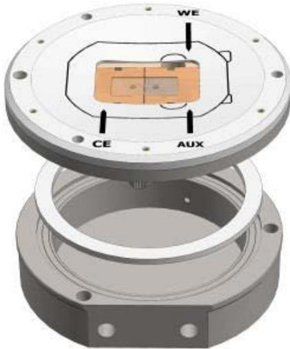
XVIII) Place the cell lid with the inner cell attached onto the cell base.
