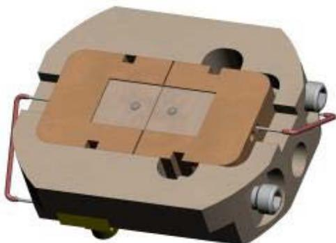
If the height of the electrodes varies, you have different means to adjust the electrodes. There are 4 adjustment screws at the inner cell.
