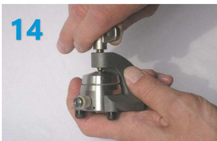
Tighten cell by turning the wing nut.
