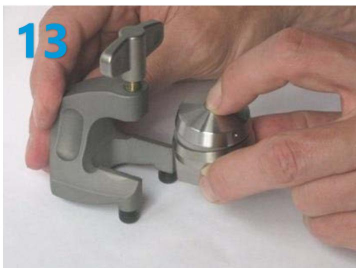
Insert the cell into the bracket by pressing down the lid while pushing the cell into the bracket.
