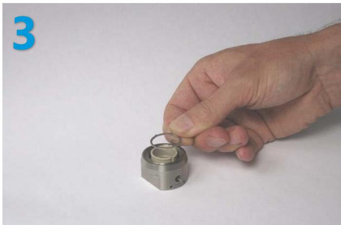
Mount the locking washer to align the side opening of the cell base with the feed-through hole of the REF sleeve.
