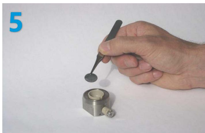
Place the 18 mm counter electrode into the sleeve.
