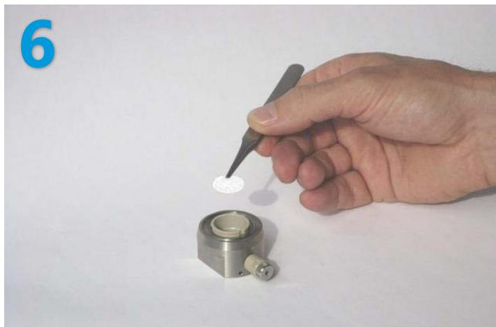
Put the glass fiber separator on top.
