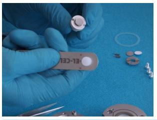
6. Use the loading tweezers to push the piston into the sleeve.
