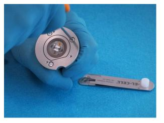
17. Finally fix the lid by using the torx screws and the hexagon screw driver 2.5mm.
