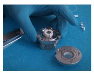
7. Place the assembly into the cell base.
