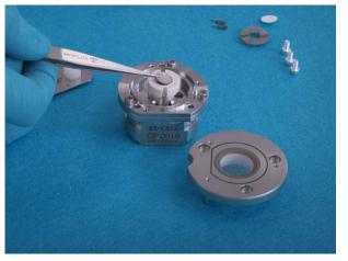
10. Put the R electrode disc, lithium metal in this case, on top of the piston.
