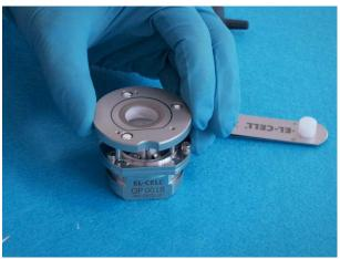
16. Use the straight marking on the lid to align it to the flat side of the cell base and attach it.
