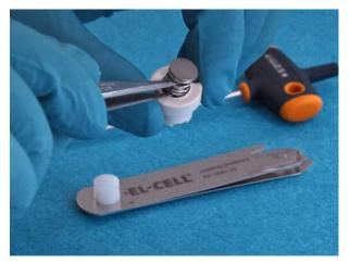
5. Insert the lower piston into the inner sleeve.
