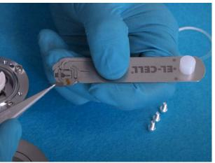
8. Insert the sample holder into the loading tweezers. Squeeze the tweezers together to lift the sample holder bracket. Then attach the first electrode strip to the sample holder.
