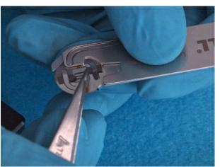
9. Turn the sample holder around and place the second electrode strip.
