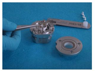
13. Attach the sample holder to the assembly. The markings 1 and 2 on sample holder and cell base represent the electrodes. Use them as an aid for correct placement.
