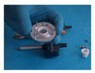
3. Insert the window thrust ring.
