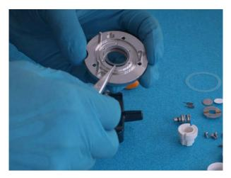
1.Turn the lid upside down. Insert the foil sealing into the lid.
