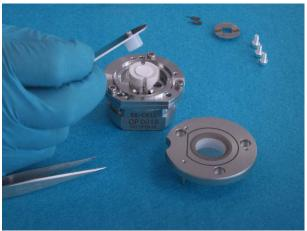
12. Use the loading tweezers again to press the cell stack further into the piston.
